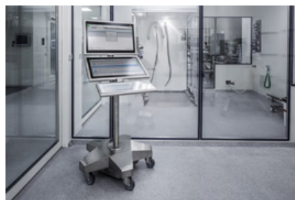
Figure 4: Mobile HMI with dual-screen display for viewing several applications at once.
