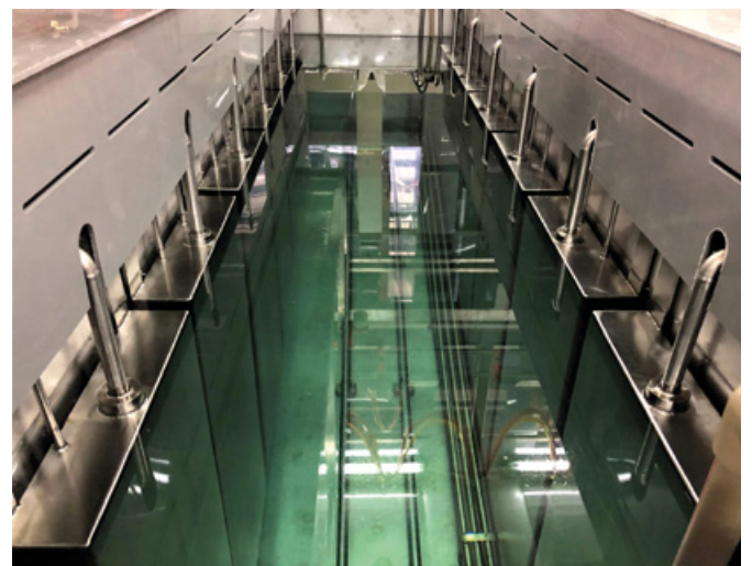
Each cleaning tank is equipped with twelve submersible transducers with 25 kHz. (Image source: Weber Ultrasonics AG)
