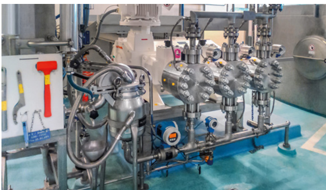
The type G3F triplex process diaphragm pump features completely safe start-up and fulfills the stringent hygienic provisions of the food industry. (Source: DSM Nutritional Products GmbH)
