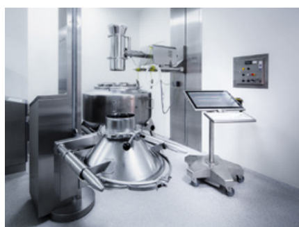
Figure 3: Mobile HMI with powerful battery in base.
