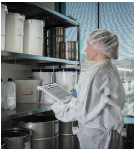
Figure 6: A tablet is particularly suitable for use in maintenance and commissioning, and for producing standard operation procedures (SOP) in cleanrooms.
