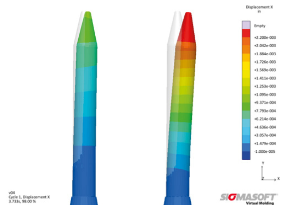
Figure 1 – Simulative comparison of the deformation of core pins made of tungsten carbide (left) and 420 stainless steel (right) at the end of the filling of the cavity – the material with the lower modulus of elasticity deforms three times more under constant process conditions.
