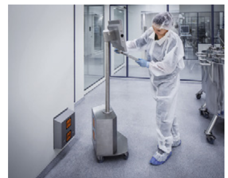
Figure 5: Inductive charging eliminates the need for cables in a cleanroom. The device can be operated while it is being charged.
