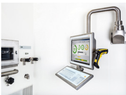
Figure 2: On-wall assembly using U-pipe support arm. Several rotatable couplings enable the HMI and support arm to rotate by 35°. The cables are routed internally as per cleanroom requirements.
