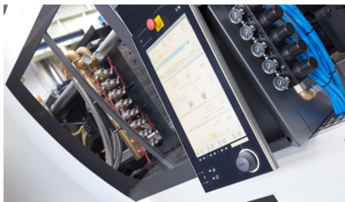
Integrated into the CC300 control of the e-motion injection molding machine, the iQ assistance systems compensate for process fluctuations in real time. (Image: ENGEL)
