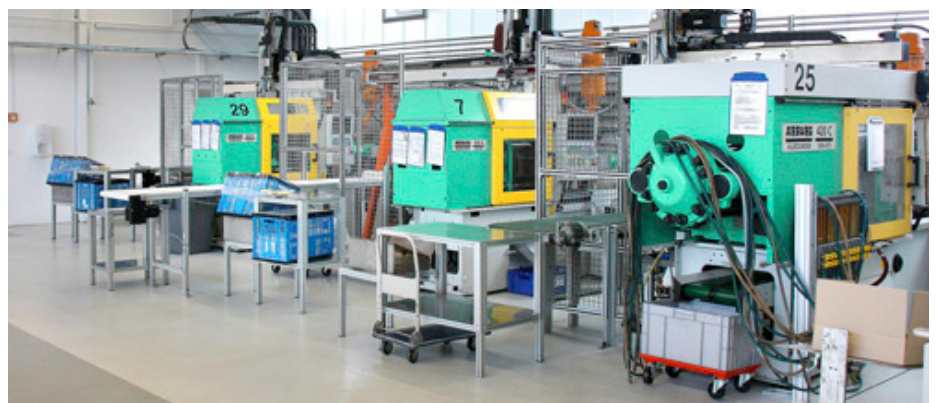
The components of the stool sampling tubes are produced on Allrounders in a SaS2 clean room. (Photo: Maier + Partner)
