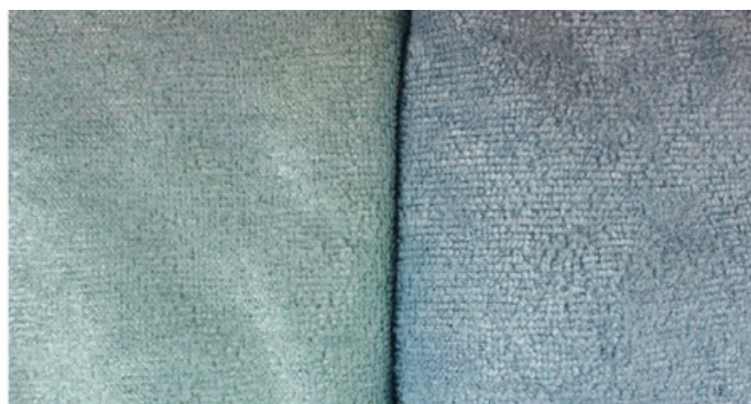
Fig. 2: Colour differences in cleaning cloths made of microfibres before and after finishing with copper pigments. ©Hohenstein Institute
