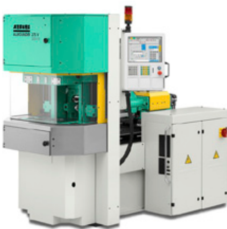
At the Chinaplas, the Hotmelt process for overmoulding electronic components will be demonstrated on a vertical Allrounder 275 V. (Photo: Arburg)
