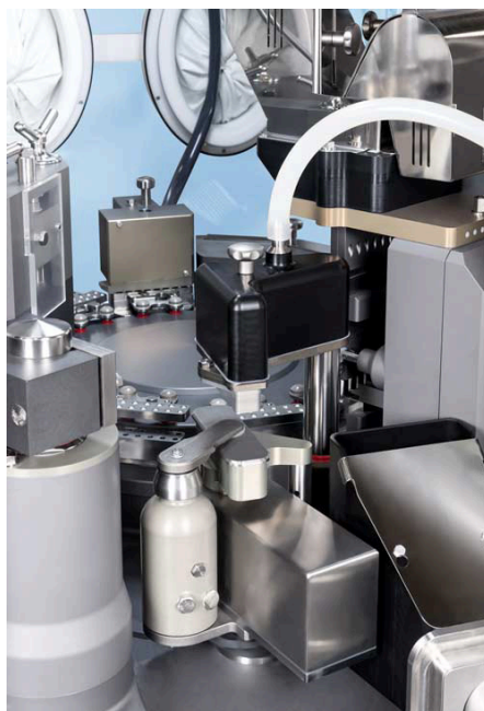
Premiere: Bosch GKF 2600 with integrated weighing station. The integrated Net Weight Detection System (NWDS) automatically corrects deviations in the filling volume for micro dosing and pellet filling. (Photo: Bosch)
