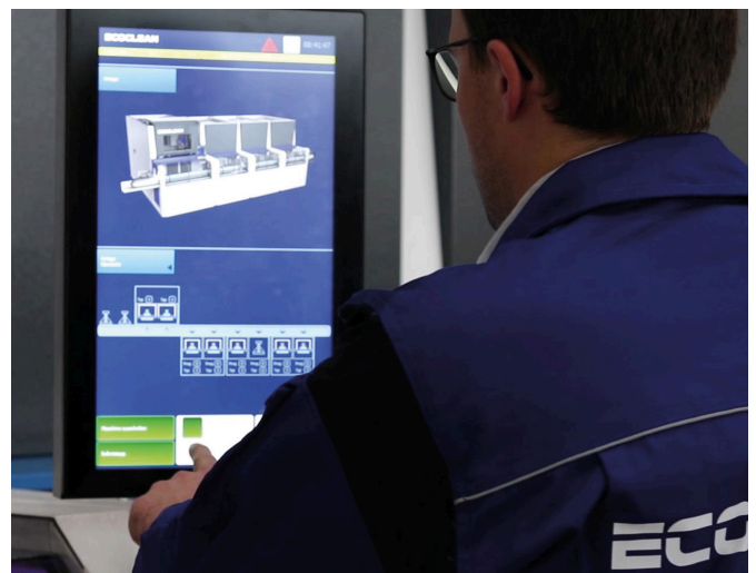
On the 19" flat screen monitor (HMI), all of the system's modules are presented separately and clearly in a complete overview diagram, similar to a smartphone display.
