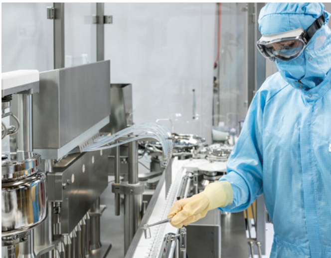
Bosch ALF 5000 for a maximum of flexibility: In the combi configuration, the ALF 5000 filling and closing machine not only processes ampoules but also injection bottles. (Picture: Bosch)
