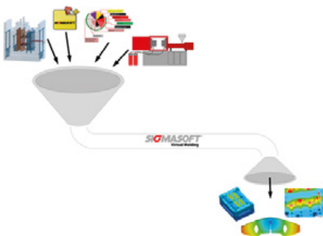
Figure 1 - With conventional approaches for injection molding simulation the user provides a combination of geometries, materials and process set-up and receives a result for this specific point inside the process window.
