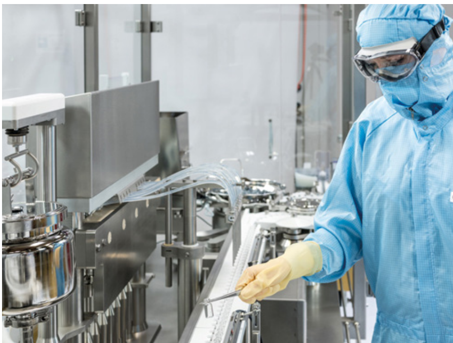
Machines and lines in action: The traditional plant tour focuses on new technologies for liquid pharmaceutical processing, including the ALF 5000 filling and closing machine ALF 5000 with a Virtual Reality application for training purposes. (Picture: Bosch)
