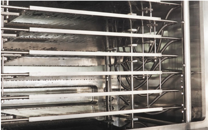
Bosch freeze dryer with tilting shelves: Fast cleaning: the slight tilt enables water droplets to quickly drain from the surface, shortening the cleaning and drying time. (Picture: Bosch)
