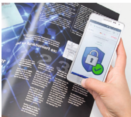
The ((rfid))-Digital Void Label enables smartphone-based electronic first-opening indication.
