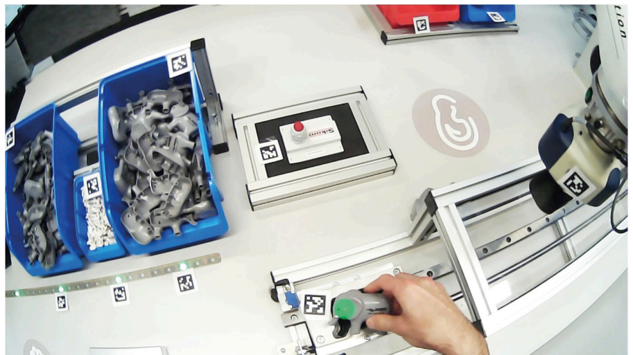
The eye-tracking systems show which areas of the workplace fitters look at for longer, which they only glance at and which they do not observe at all. (© Fraunhofer IPA)
