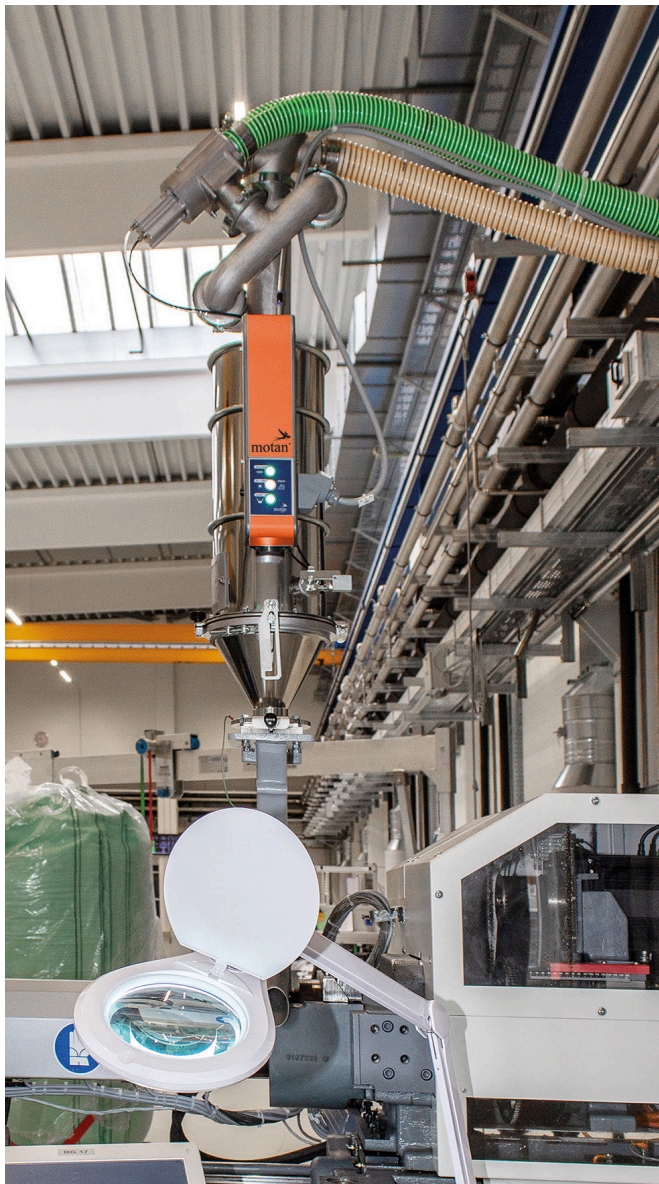
De-dusting modules enable the use of regrind without loss of quality. The dust is automatically separated into the central filter in a separate room. (Image: motan-colortronic)
