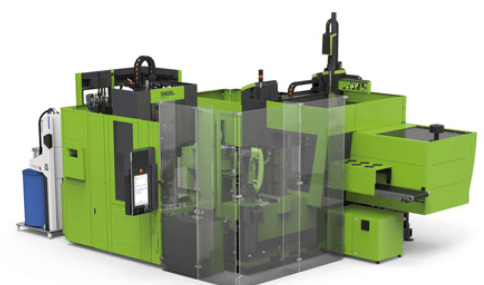
For the production of two-component housing demo parts at the K show, ENGEL is combining a victory 120 AMM with an insert 60V/45 vertical injection moulding machine. (Picture: ENGEL)
