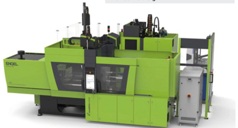
Premiere for the two-component AMM process. A silicone seal is directly moulded onto the parts, which are made of amorphous metal. (Picture: ENGEL)
