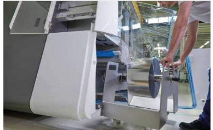
Foil rolls can be replaced on the fly without needing to stop the machine. (Source: Mediseal GmbH)
