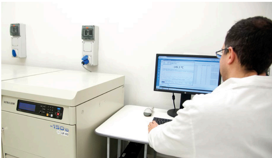
Dr. Motta checking the status of a cryogenic freezer in a viewLinc pop-up alarm window.
