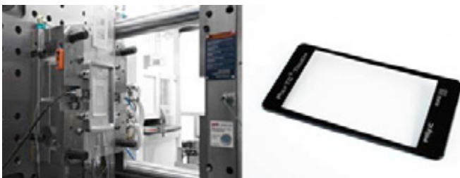
On the clamping side of the mould the frame of the 5" display is decorated using the IMD unit directly during injection.
