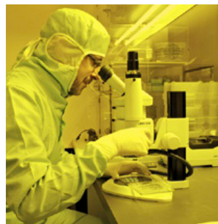
On the light microscope, Helmut Schift checks whether the stamp structures have been moulded evenly during the thermal imprint and whether process changes are necessary. (Photo: Paul Scherrer Institute/Markus Fischer)
