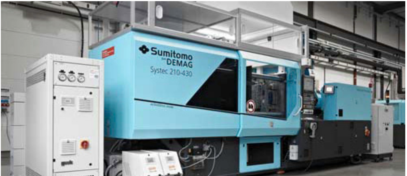
Compact production cell with a Systec 210 combining IML and IMD technology. A multi-touch-capable display is produced here in one shot.
