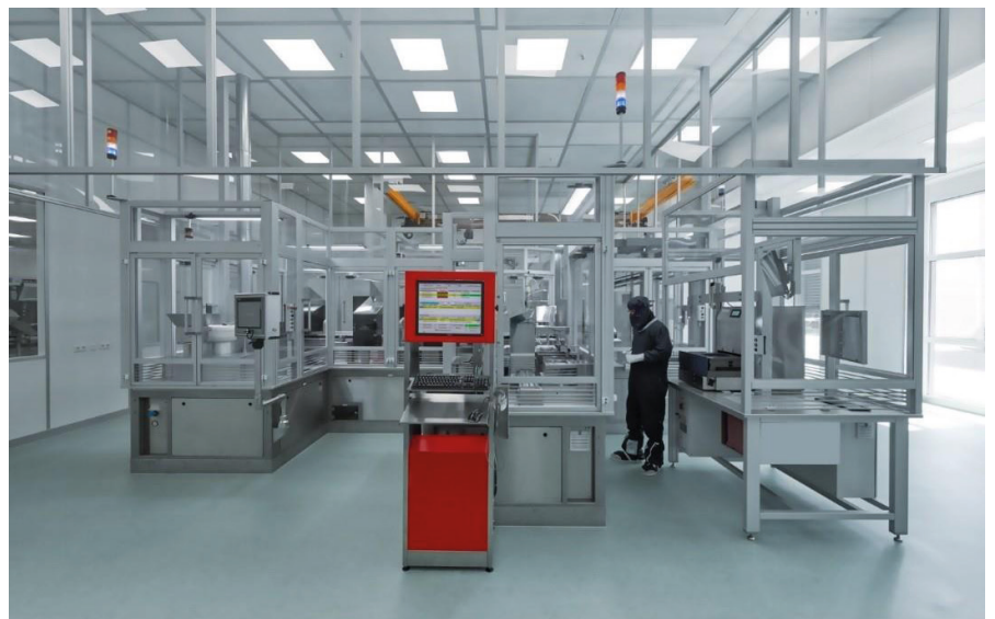
Production in the clean room according to GMP Grade C of the pre-fillable plastic syringe with cannula.
