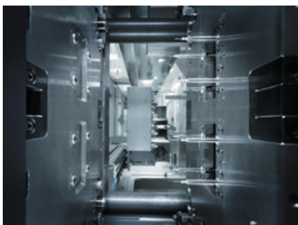
The cannula is insert-molded during the injection molding procedure. The syringe is free of tungsten and glue.
