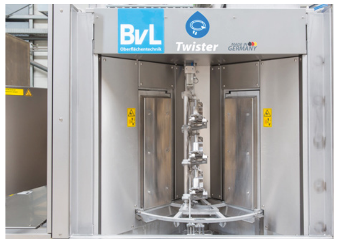
Three throttle valves that need to be cleaned are placed by robots on specially manufactured workpiece holders and rotated through the treatment chambers as part of the automatic cycle mode.
