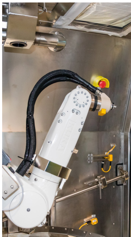
The inner walls are made of electropolished stainless steel, thus ensuring extremely smooth and easy-to-clean surfaces. (Photo source: acp systems AG)
