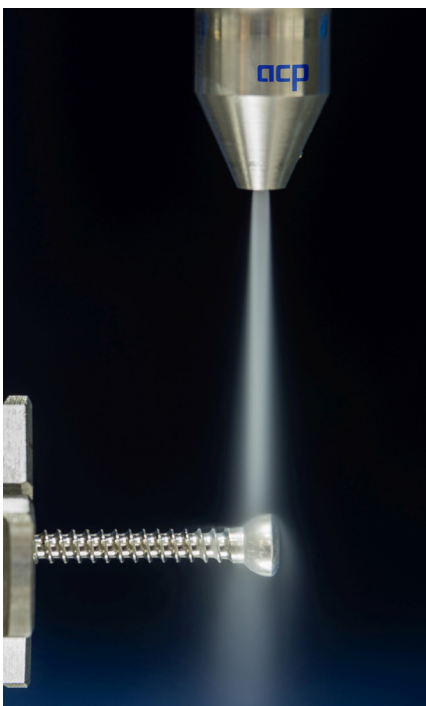
The quattroClean system, which can be integrated into networked manufacturing environments, enables the partial or full-surface removal of particulate and filmic contamination from practically all technical materials in clean environments. (Photo source: acp systems AG)
