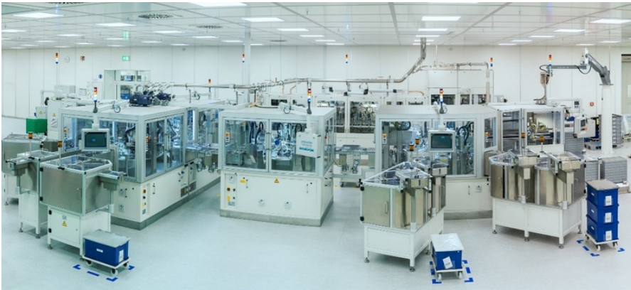
High-volume line for the assembly of the Respimat® reusable inhaler housing module in a clean-room ISO class 8 in Pfreimd, Germany.
