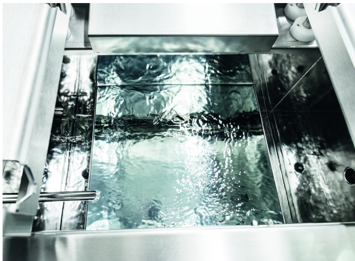
All wet-stage tanks of the system, which is entirely made from electropolished stainless steel, have a two-sided overflow which ensures the immediate removal of detached particles and other contaminants. This minimizes the risk of recontamination when the parts are moved. (Image source: UCM AG)
