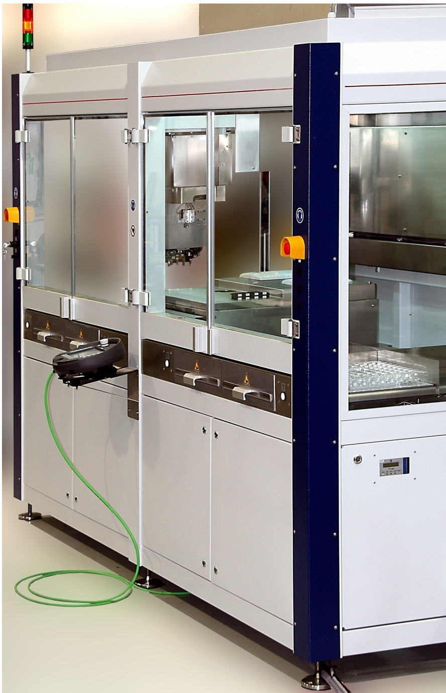
To clean sensors, the CO 2 snow jet system was integrated into a standard module featuring a clean air supply and a media preparation system for the liquid carbon dioxide and compressed air. (Photo source: acp systems AG)
