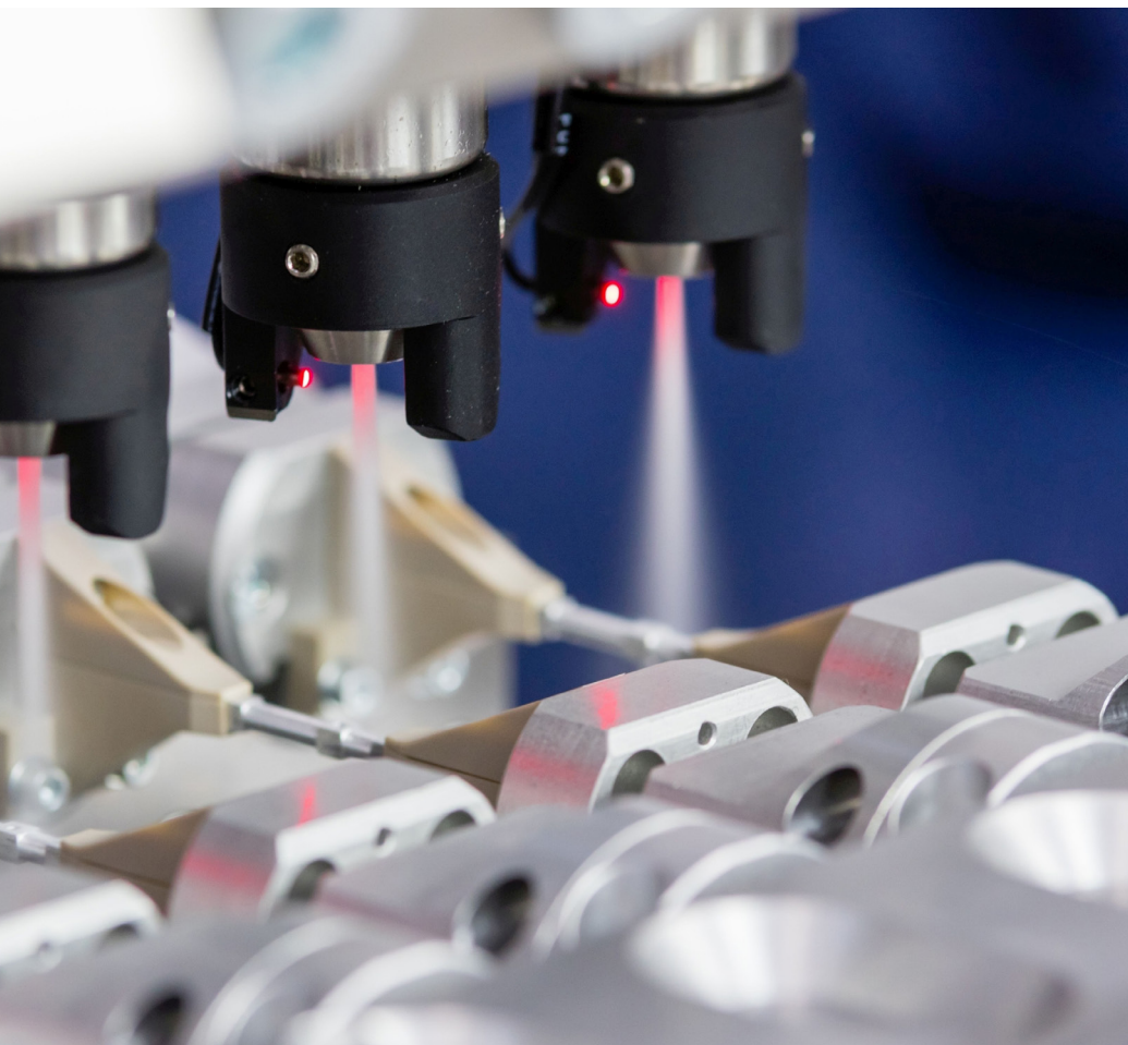
The quality of the cleaning jet can be monitored with sensors and converted into a digital value which is assigned to each individual part and then stored and documented. (Photo source: acp systems AG)
