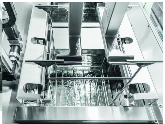
Up to nine cleaning and rinsing steps can be integrated into the cleaning system and variably equipped for use with single, dual and multi-frequency ultrasonics.
