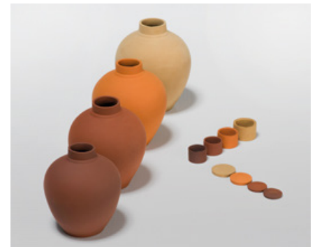
Vases, rings, and tablets made from simulated Martian soil in various stages of firing. (© TU Berlin/David Karl)
