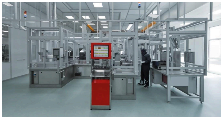
Production in the clean room according to GMP Grade C of the pre-fillable plastic syringe with cannula.
