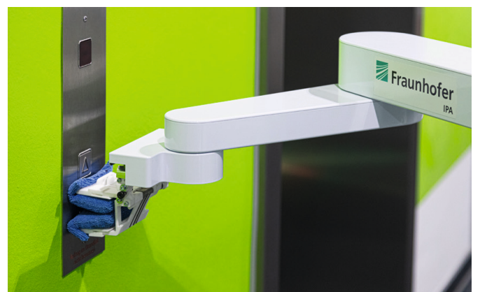
By using its flexible cleaning tool, DeKonBot can disinfect different objects by wiping, including elevator buttons. (© Fraunhofer IPA/Photo: Rainer Bez)
