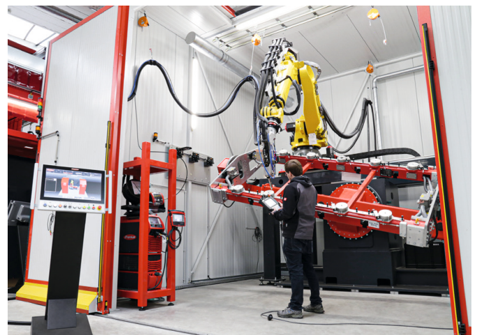
The LaserHybrid process ensures fast, reliable seams with low levels of distortion – especially for large components such as battery trays. (Photo: Fronius International GmbH)
