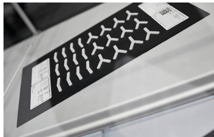
The company Samaplast has used a Freeformer 200-3X and APF to process absorbable original materials into bone-like implants. (Photo: Arburg)
