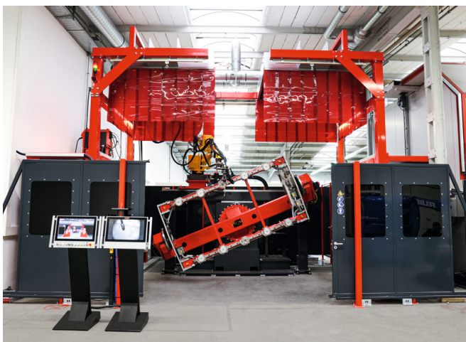
The robot welding cells in the Fronius prototyping centre are equipped with the latest clamping, sensor, and welding technology – such as the CMT process. (Photo: Fronius International GmbH)
