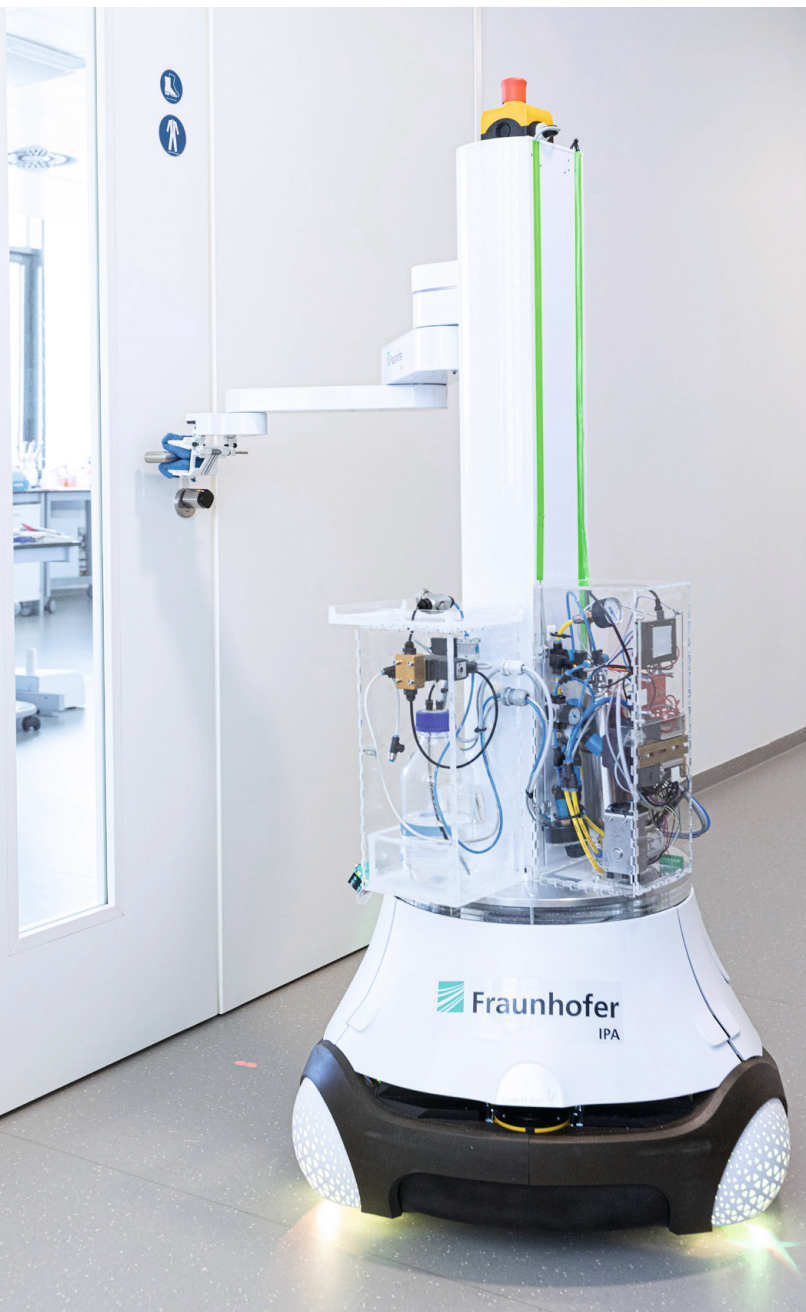
The mobile cleaning and disinfection robot DeKonBot navigates autonomously to critical objects such as door handles and disinfects them. (© Fraunhofer IPA/Photo: Rainer Bez)
