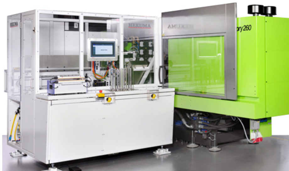
Together with its system partner Hekuma, ENGEL has created a high-speed automation to produce the petri dishes. (Picture: Hekuma)
