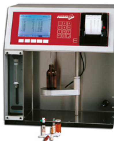
The PAMAS SVSS particle counting system measures infusion solutions, parenterals, intravenous or ophthalmic liquids and further pharmaceutical suspensions in compliance with the US pharmacopoeia. The measuring results are reported with the help of the pharmaceutical procedural software PAMAS USP. With the aid of a Small Volume Kit (accessory for small volume samples), the instrument can now be used to analyse Therapeutic Protein Injections as per USP 787. (Picture: PAMAS)
