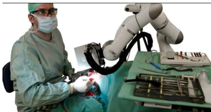
Robot CARLO (Computer Assisted Robot-guided Laser Osteotome) cuts bones contactless and highly accurately. (Photo: AOT AG Basel)
