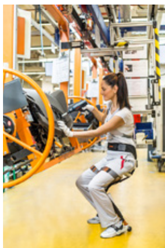
The Chairless Chair facilitates many activities in assembly. This high-tech construction made of carbon lets Audi employees sit without any chair. At the same time, it helps to improve posture and reduces leg strain. (Photo: Audi)
