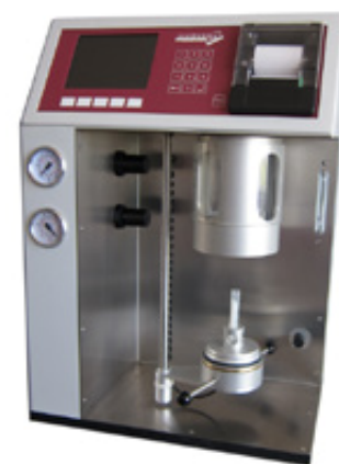
The particle analysing system PAMAS SBSS may be optionally equipped with a small pressure container. With the help of this feature, smallest sample volumes of higher viscosity, like Therapeutic Protein Injections, can be analysed as per USP 787. (Picture: PAMAS)
