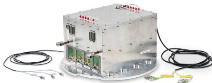
MAIUS laser system: Used to successfully create a Bose-Einstein condensate for the first time in space. It is about as big as a shoe box with a mass of 27 kg. FBH's laser modules are integrated on the bottom side of the heat sink, the top side houses modules for further processing of the light to be transferred to the main experiment. (© Humboldt-Universitaet zu Berlin)
