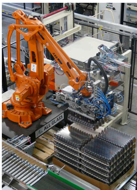
The robot arm puts a layer of shrink wrapped bottles on the pallet.
