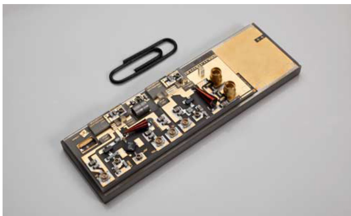
MOPA laser module for MAIUS: Hybrid-integrated master-oscillator power-amplifier (MOPA) laser module for rubidium precision spectroscopy in space developed by the Ferdinand-Braun-Institut – three of these MOPA modules along with two redundant modules are integrated into the laser system. (© FBH/schurian.com)
