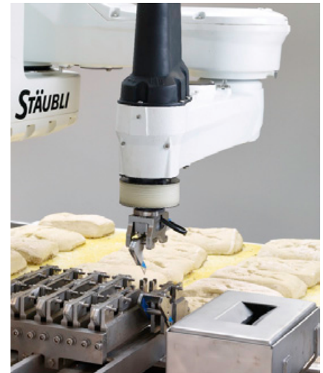
TP80 seen here slicing baked goods with a cycle time of 220 cuts per minute.
