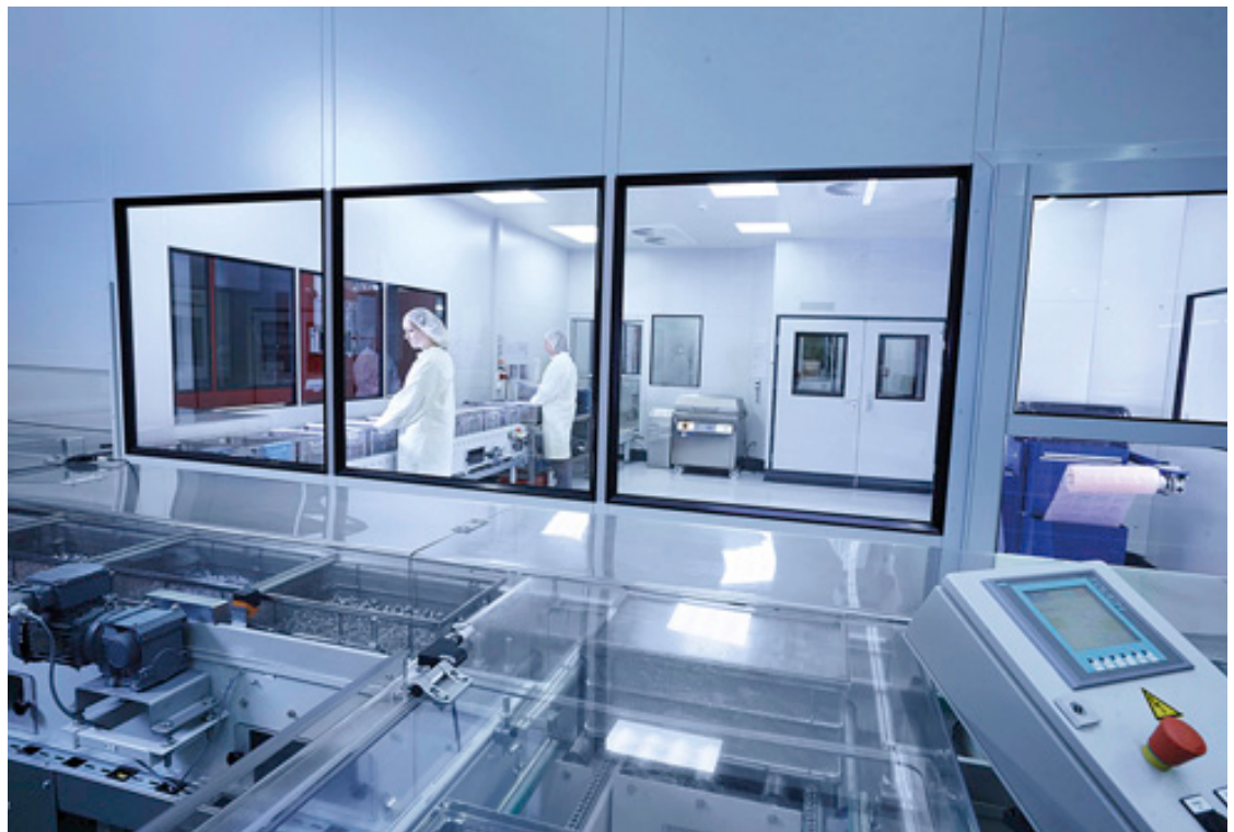
Clean room in the EJOCLEAN® Centre - the goods are packed in a clean room in order to prevent re-contamination through air-borne particles.
