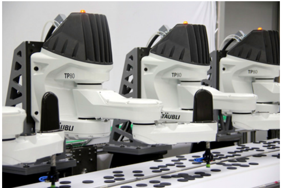
TP80 production line for highly complex sorting and packaging tasks.
