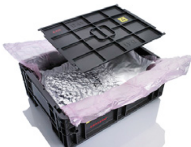
Vacuum packed screws in a small load carrier protected against shocks during transport by air bubble film.
