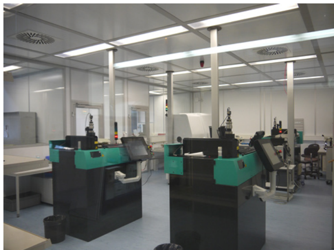
Another ISO class 8 clean room with laser cutting systems for the precision machining of stainless steel pipes for manufacturing stents.
