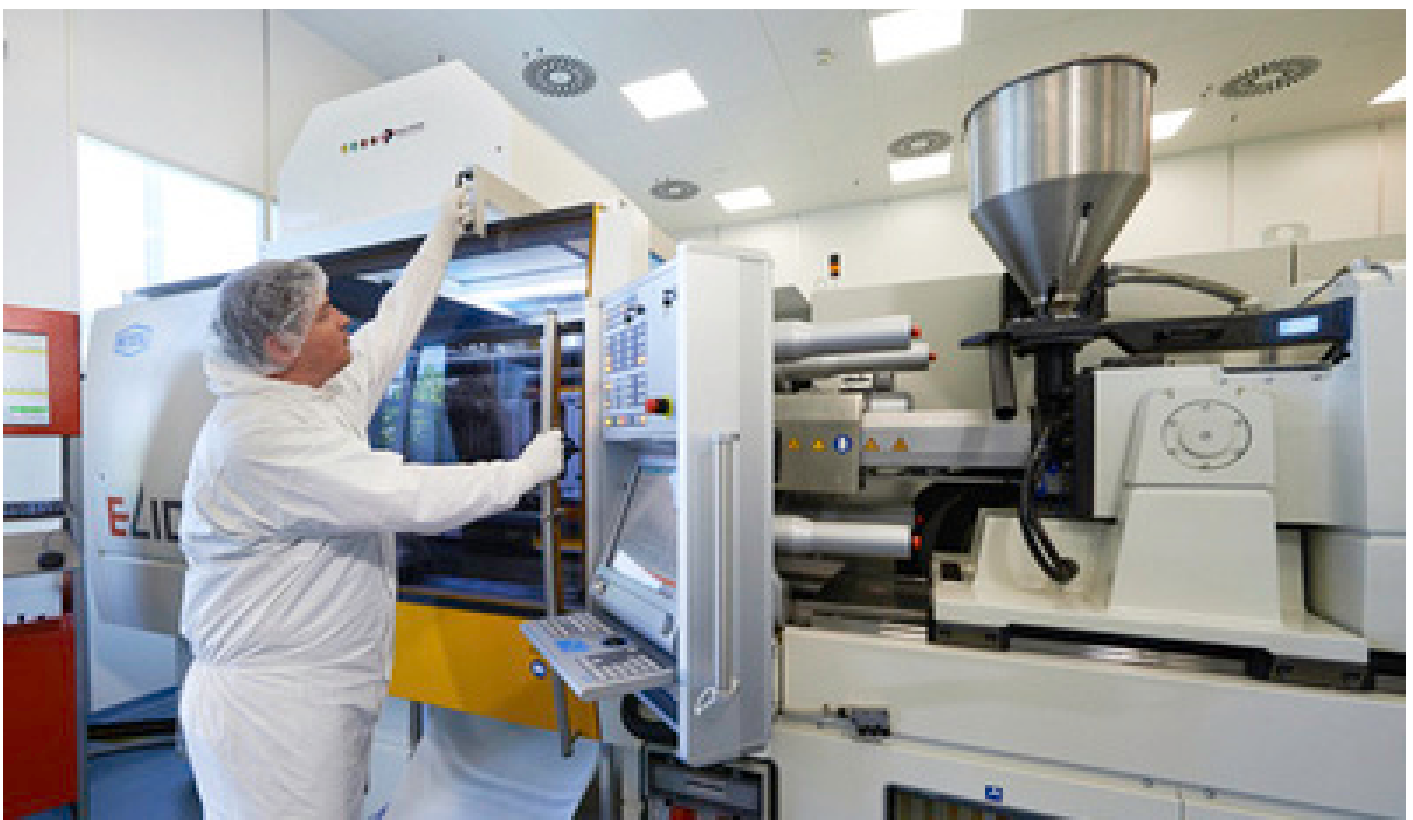
Integrated laminar flow hoods create an ISO class 7 cleanroom environment in the injection molding area.
