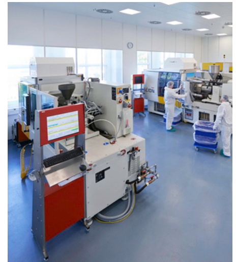
Pilot production in a class 8 cleanroom to DIN EN ISO 14644 standard at the Technical Competence Center in Wackersdorf.
