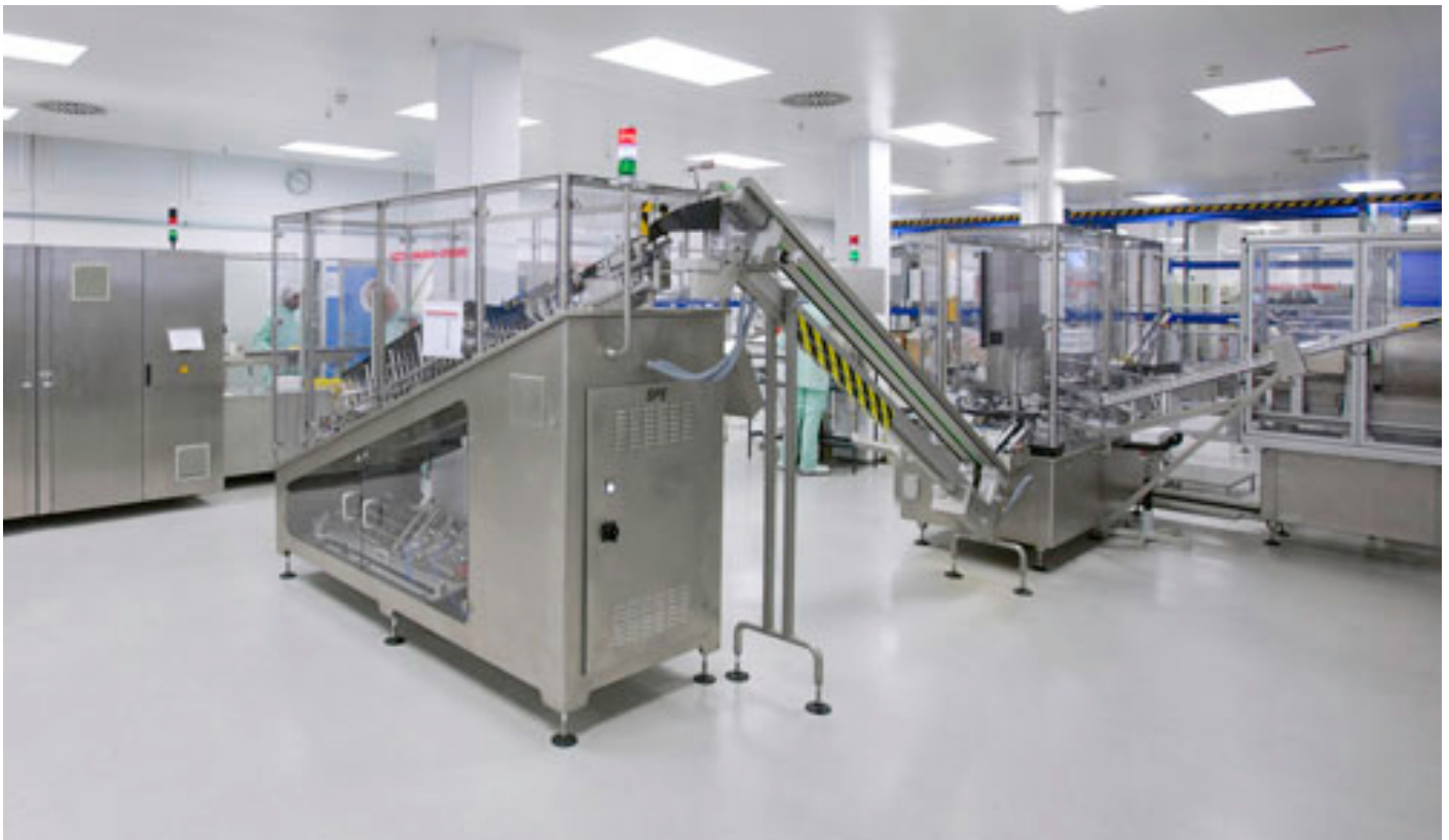
Figure 5: All from a single source: Compact, fully automatic production systems cut costs. On this syringe line, plunger assembly, labelling, safety device assembly and syringe buffering dovetail intelligently. (Photo: Bausch + Ströbel)
