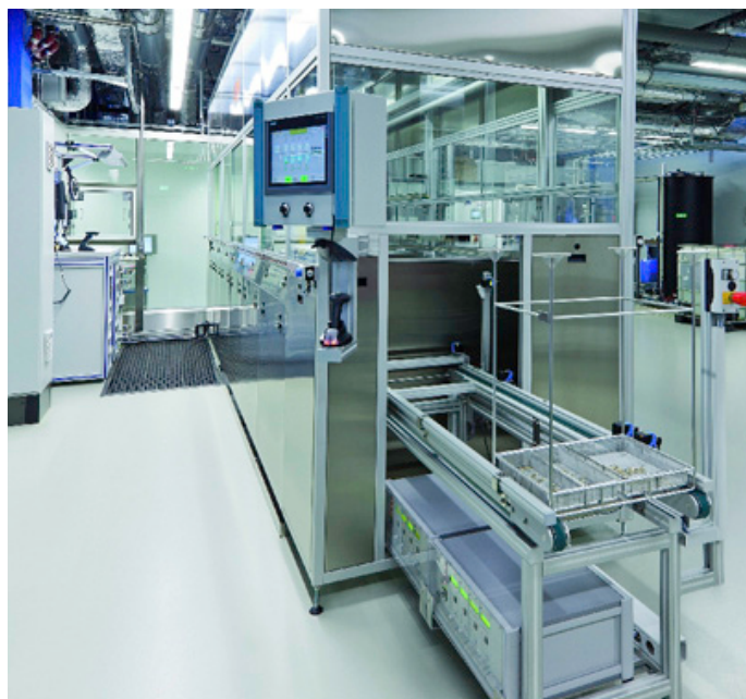
The final cleaning system delivers the product directly into the cleanroom. The system and its conveyor unit are fully enclosed all the way into the cleanroom.
