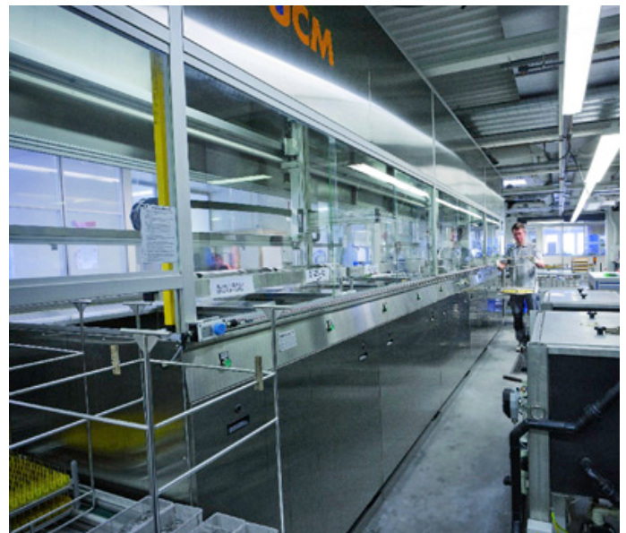
The first stage of the ultrasonic cleaning system used for final cleaning has three separate tanks. Parts consisting of different materials can thus be cleaned separately.
