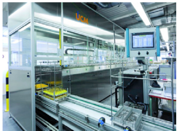
The equipment controller stores 16 different programs for final cleaning of the diverse parts.
