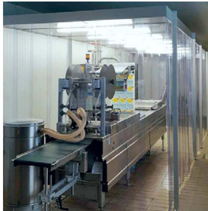
Packing of organic spread. CleanFlowCell® laminar flow housing, clean room class ISO-7.
