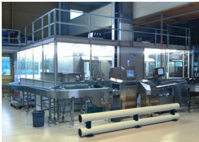
Packing sliced bread in a large-scale bakery. The CleanSteriCell® closed system in clean room class ISO-7 meets requirements for pharmaceutical production.
