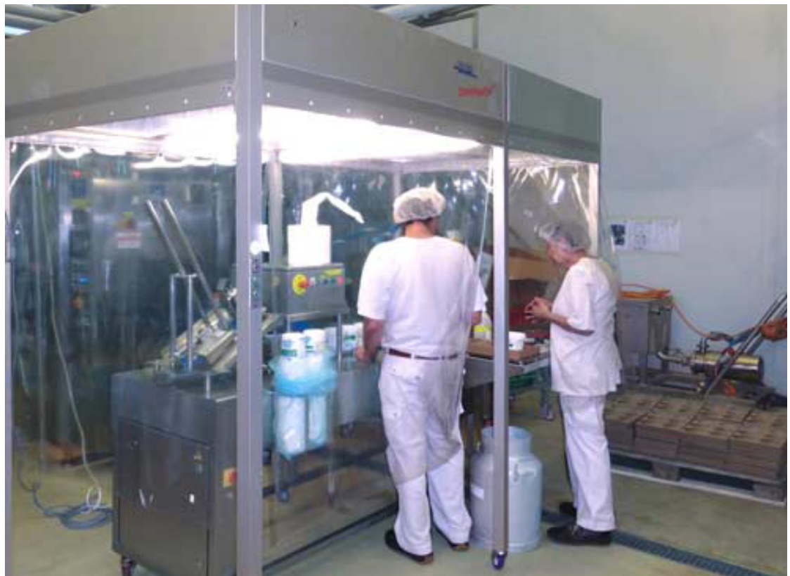
Organic yoghurt filling process. CleanFlowCell® laminar flow housing, clean room class ISO-7.
